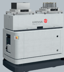
AGVs can be integrated for de- livering/returning tools and workpieces
