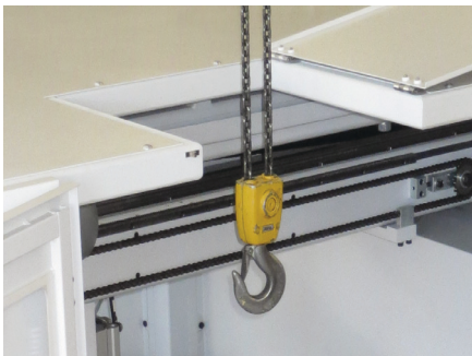
Top loading door for crane operation.
