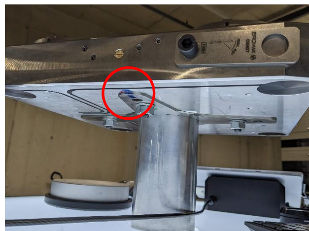
Figure 6: Base plate orientation and mounting 4 x M12
